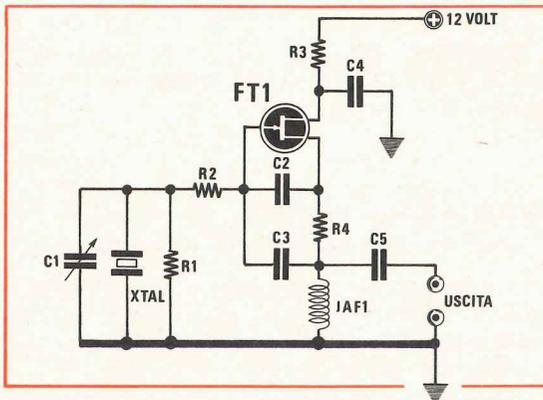
**Fig. 9 OSCILLATORE A FET in FONDAMENTALE (4 MHz a 20 MHz)**
